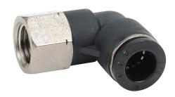
NITRA pneumatic push-to-connect fitting, elbow, rotating, thermoplastic (PBT) body, nickel-plated brass threads, (1) 1/4in female NPT to (1) 3/8in push-to-connect. Package of 5.
