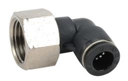
NITRA pneumatic push-to-connect fitting, elbow, rotating, thermoplastic (PBT) body, nickel-plated brass threads, (1) 1/2in female NPT to (1) 3/8in push-to-connect. Package of 5.
