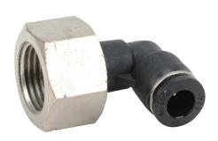
NITRA pneumatic push-to-connect fitting, elbow, rotating, thermoplastic (PBT) body, nickel-plated brass threads, (1) 3/8in female NPT to (1) 1/4in push-to-connect. Package of 5.
