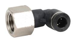
NITRA pneumatic push-to-connect fitting, elbow, rotating, thermoplastic (PBT) body, nickel-plated brass threads, (1) 1/4in female NPT to (1) 1/4in push-to-connect. Package of 5.
