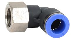
NITRA pneumatic push-to-connect fitting, elbow, rotating, thermoplastic (PBT) body, nickel-plated brass threads, (1) R3/8 female BSPT to (1) 12mm push-to-connect. Package of 5.
