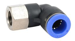
NITRA pneumatic push-to-connect fitting, female, elbow, rotating, thermoplastic (PBT) body, nickel-plated brass threads, 12mm tube to R1/4 BSPT connection(s). Package of 5.
