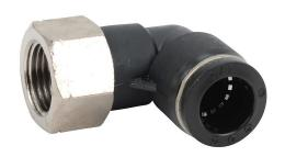
NITRA pneumatic push-to-connect fitting, elbow, rotating, thermoplastic (PBT) body, nickel-plated brass threads, (1) 3/8in female NPT to (1) 1/2in push-to-connect. Package of 5.
