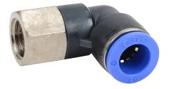
NITRA pneumatic push-to-connect fitting, elbow, rotating, thermoplastic (PBT) body, nickel-plated brass threads, (1) R1/4 female BSPT to (1) 10mm push-to-connect. Package of 5.
