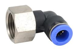
NITRA pneumatic push-to-connect fitting, elbow, rotating, thermoplastic (PBT) body, nickel-plated brass threads, (1) R1/2 female BSPT to (1) 10mm push-to-connect. Package of 5.
