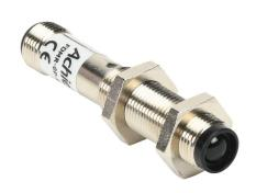
AchieVe photoelectric sensor, tubular, threaded, metal housing, through-beam receiver, 4m sensing distance, 10-30 VDC operating voltage, selectable light-on/dark-on, PNP, 4-wire, 4-pin M12 quick-disconnect.
