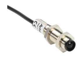
AchieVe photoelectric sensor, tubular, threaded, metal housing, through-beam receiver, 4m sensing distance, 10-30 VDC operating voltage, selectable light-on/dark-on, PNP, 4-wire, pigtail.
