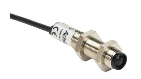
AchieVe photoelectric sensor, tubular, threaded, metal housing, through-beam emitter, infrared, 4m sensing distance, 10-30 VDC operating voltage, 3-wire, pigtail.
