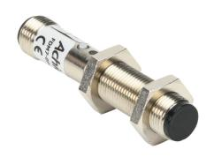
AchieVe photoelectric sensor, tubular, threaded, diffuse, infrared, 300mm sensing distance, selectable light-on/dark-on, PNP, teachin button, 1 kHz switching frequency, metal housing, 4-pin M12 quick-disconnect.
