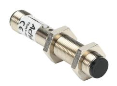
AchieVe photoelectric sensor, tubular, threaded, diffuse, infrared light emission, 300mm sensing distance, selectable light-on/dark-on, PNP, teach-in button, 1 kHz switching frequency, metal housing, 4-pin M12 quick-disconnect.
