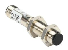
AchieVe photoelectric sensor, tubular, threaded, diffuse, infrared, 300mm sensing distance, selectable light-on/dark-on, NPN, teachin button, 1 kHz switching frequency, metal housing, 4-pin M12 quick-disconnect.
