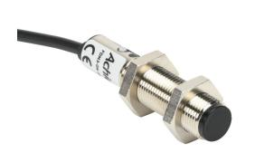
AchieVe photoelectric sensor, tubular, threaded, diffuse, infrared, 100mm sensing distance, selectable light-on/dark-on, NPN, teachin button, 1 kHz switching frequency, metal housing, pigtail.
