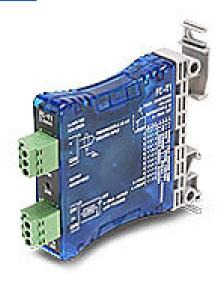
AutomationDirect temperature transmitter, isolated, thermocouple or millivolt input, deg F or deg C, 4-20 mA output, 24 VDC operating voltage, 35mm DIN rail or panel mount, removable screw terminal plugs.
