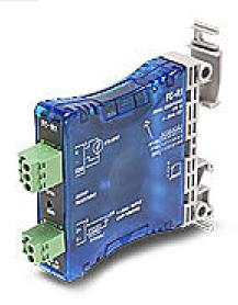
AutomationDirect temperature transmitter, isolated, RTD input, deg F or deg C, 4-20 mA output, 24 VDC operating voltage, 35mm DIN rail or panel mount, removable screw terminal plugs.
