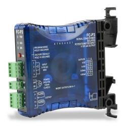
Signal conditioner, isolated, potentiometer input, current or voltage output, 24 VAC/VDC operating voltage, 35mm DIN rail or panel mount, removable screw terminal plugs.
