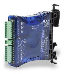
AutomationDirect signal conditioner, isolated, differential or single ended line driver input, differential line driver output, 24 VDC operating voltage, 35mm DIN rail or panel mount, removable screw terminal plugs.
