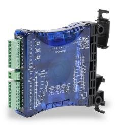
AutomationDirect signal conditioner, isolated, differential or single ended line driver input, open collector output, 7.8-24 VDC operating voltage, 35mm DIN rail or panel mount, removable screw terminal plugs.
