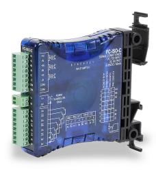
Signal conditioner, isolated, differential or single ended line driver input, open collector output, 7.8 to 24 VDC operating voltage, 35mm DIN rail or panel mount, removable screw terminal plugs.
