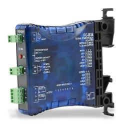
Signal conditioner, isolated, bi-polar voltage input, current or voltage output, 24 VDC operating voltage, 35mm DIN rail or panel mount, removable screw terminal plugs.
