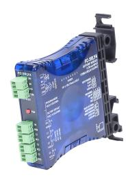
AutomationDirect limit alarm, current or voltage input, (4) SPST relay output, 24 VAC/VDC operating voltage, 35mm DIN rail or panel mount, removable screw terminal block(s).
