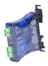
Limit alarm, current, voltage input, (2) SPDT relay output, 24 VAC/ VDC operating voltage, 35mm DIN rail or panel mount, removable screw terminal block(s).
