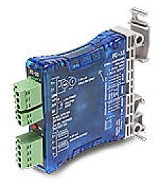
Signal conditioner, isolated, current or voltage input, current or voltage output, 24 VDC operating voltage, 35mm DIN rail or panel mount, removable screw terminal plugs.
