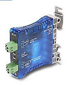
Signal conditioner, isolated, current input, current output, 24 VDC operating voltage, 35mm DIN rail or panel mount, removable screw terminal plugs.
