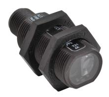
AutomationDirect photoelectric sensor, tubular, threaded, plastic housing, through-beam receiver, 8m sensing distance, 10-30 VDC operating voltage, light-on, PNP, 3-wire, 4-pin M12 quick-disconnect.
