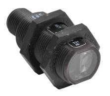
AutomationDirect photoelectric sensor, tubular, threaded, plastic housing, through-beam receiver, 8m sensing distance, 10-30 VDC operating voltage, light-on, NPN, 3-wire, 4-pin M12 quickdisconnect.
