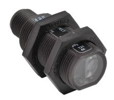
AutomationDirect photoelectric sensor, tubular, threaded, plastic housing, through-beam receiver, 8m sensing distance, 10-30 VDC operating voltage, dark-on, PNP, 3-wire, 4-pin M12 quick-disconnect.
