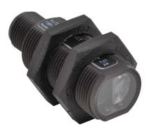
AutomationDirect photoelectric sensor, tubular, threaded, plastic housing, through-beam receiver, 8m sensing distance, 10-30 VDC operating voltage, dark-on, NPN, 3-wire, 4-pin M12 quick-disconnect.
