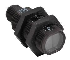
AutomationDirect photoelectric sensor, tubular, threaded, polarized retroreflective, visible red, 2.5m sensing distance, light-on, PNP, 3-wire, 4-pin M12 quick-disconnect.
