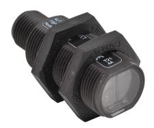
AutomationDirect photoelectric sensor, tubular, threaded, polarized retroreflective, visible red light emission, 2.5m sensing distance, light-on, NPN, 3-wire, 4-pin M12 quick-disconnect.
