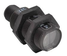
AutomationDirect photoelectric sensor, tubular, threaded, polarized retroreflective, visible red, 2.5m sensing distance, light-on, NPN, 3-wire, 4-pin M12 quick-disconnect.
