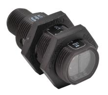
AutomationDirect photoelectric sensor, tubular, threaded, polarized retroreflective, visible red, 2.5m sensing distance, darkon, PNP, 3-wire, 4-pin M12 quick-disconnect.
