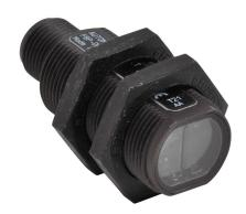
AutomationDirect photoelectric sensor, tubular, threaded, polarized retroreflective, visible red light emission, 2.5m sensing distance, dark-on, NPN, 3-wire, 4-pin M12 quick-disconnect.
