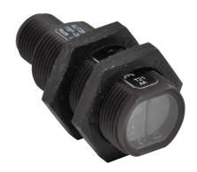
AutomationDirect photoelectric sensor, tubular, threaded, polarized retroreflective, visible red, 2.5m sensing distance, darkon, NPN, 3-wire, 4-pin M12 quick-disconnect.
