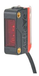
AchieVe photoelectric sensor, rectangular, polarized retroreflective, visible red, 0.02–5m sensing distance, selectable light-on/dark-on, NPN, potentiometer, 3-wire, pigtail.
