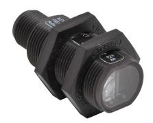
AutomationDirect photoelectric sensor, tubular, threaded, plastic housing, through-beam emitter, visible red light emission, 8m sensing distance, 10-30 VDC operating voltage, 2-wire, 4-pin M12 quick-disconnect.
