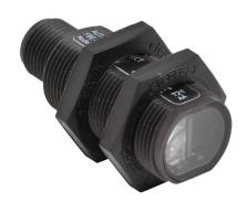
AutomationDirect photoelectric sensor, tubular, threaded, plastic housing, through-beam emitter, visible red, 8m sensing distance, 10-30 VDC operating voltage, 2-wire, 4-pin M12 quick-disconnect.
