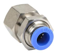
NITRA pneumatic push-to-connect fitting, bulkhead, nickel-plated brass body, nickel-plated brass threads, (1) R1/4 female BSPT to (1) 5/16in (8mm) push-to-connect. Package of 5.
