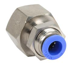
NITRA pneumatic push-to-connect fitting, bulkhead, nickel-plated brass body, nickel-plated brass threads, (1) R1/2 female BSPT to (1) 5/16in (8mm) push-to-connect. Package of 5.
