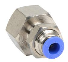
NITRA pneumatic push-to-connect fitting, bulkhead, nickel-plated brass body, nickel-plated brass threads, (1) R3/8 female BSPT to (1) 6mm push-to-connect. Package of 5.
