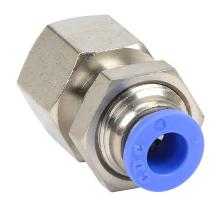
NITRA pneumatic push-to-connect fitting, bulkhead, nickel-plated brass body, nickel-plated brass threads, (1) R1/8 female BSPT to (1) 6mm push-to-connect. Package of 5.
