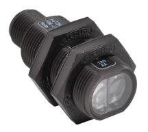
AutomationDirect photoelectric sensor, tubular, threaded, diffuse, visible red, 400mm sensing distance, light-on, PNP, potentiometer, 1 kHz switching frequency, plastic housing, 4-pin M12 quick-disconnect.
