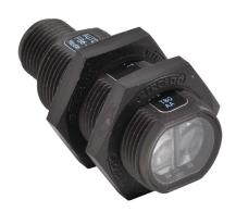
AutomationDirect photoelectric sensor, tubular, threaded, diffuse, visible red light emission, 400mm sensing distance, light-on, NPN, potentiometer, 1 kHz switching frequency, plastic housing, 4-pin M12 quick-disconnect.
