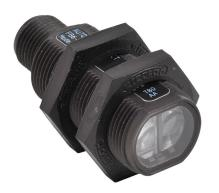
AutomationDirect photoelectric sensor, tubular, threaded, diffuse, visible red, 400mm sensing distance, light-on, NPN, potentiometer, 1 kHz switching frequency, plastic housing, 4-pin M12 quick-disconnect.
