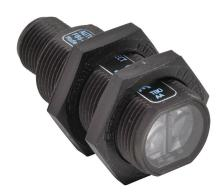
AutomationDirect photoelectric sensor, tubular, threaded, diffuse, visible red, 400mm sensing distance, dark-on, NPN, potentiometer, 1 kHz switching frequency, plastic housing, 4-pin M12 quick-disconnect.
