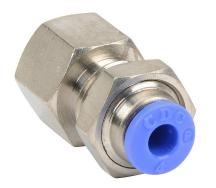
NITRA pneumatic push-to-connect fitting, bulkhead, nickel-plated brass body, nickel-plated brass threads, (1) R1/8 female BSPT to (1) 5/32in (4mm) push-to-connect. Package of 5.
