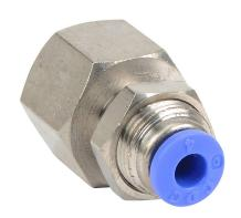
NITRA pneumatic push-to-connect fitting, bulkhead, nickel-plated brass body, nickel-plated brass threads, (1) R1/4 female BSPT to (1) 5/32in (4mm) push-to-connect. Package of 5.
