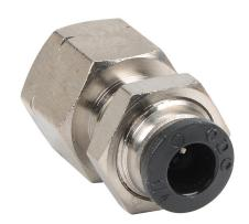
NITRA pneumatic push-to-connect fitting, bulkhead, nickel-plated brass body, nickel-plated brass threads, (1) 1/4in female NPT to (1) 1/4in push-to-connect. Package of 5.
