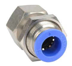
NITRA pneumatic push-to-connect fitting, bulkhead, nickel-plated brass body, nickel-plated brass threads, (1) R1/8 female BSPT to (1) 12mm push-to-connect. Package of 5.
