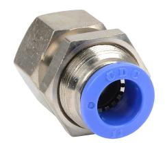
NITRA pneumatic push-to-connect fitting, bulkhead, nickel-plated brass body, nickel-plated brass threads, (1) R1/4 female BSPT to (1) 12mm push-to-connect. Package of 5.
