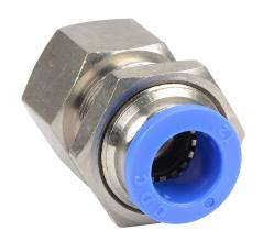
NITRA pneumatic push-to-connect fitting, bulkhead, nickel-plated brass body, nickel-plated brass threads, (1) R1/2 female BSPT to (1) 12mm push-to-connect. Package of 5.
