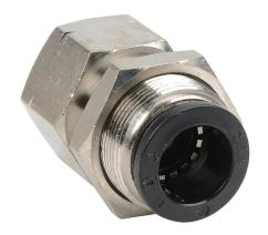
NITRA pneumatic push-to-connect fitting, bulkhead, nickel-plated brass body, nickel-plated brass threads, (1) 3/8in female NPT to (1) 1/2in push-to-connect. Package of 5.
