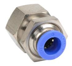
NITRA pneumatic push-to-connect fitting, bulkhead, nickel-plated brass body, nickel-plated brass threads, (1) R3/8 female BSPT to (1) 10mm push-to-connect. Package of 5.
